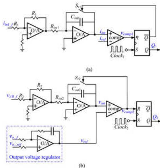
**Fig. 4. Control circuit of OCC controllers in operating mode I. (a) OCC controller of  $i_{in1}$ . (b) OCC controller of  $v_{AB}$**
