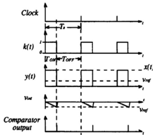
Fig.3 Waveform of one cycle controlled constant frequency switch
