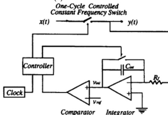
Fig.2. One cycle controlled constant frequency switch
