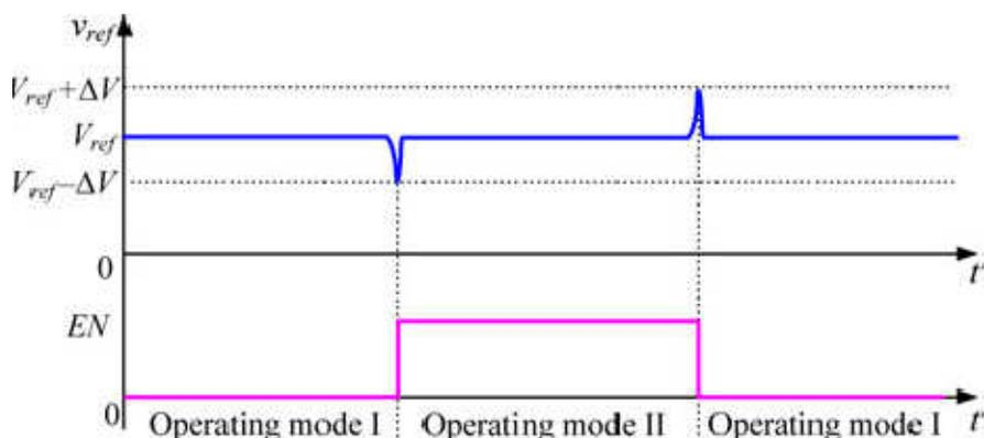
**Fig 8 Transient of  $V_{ref}$  during the mode transition**
