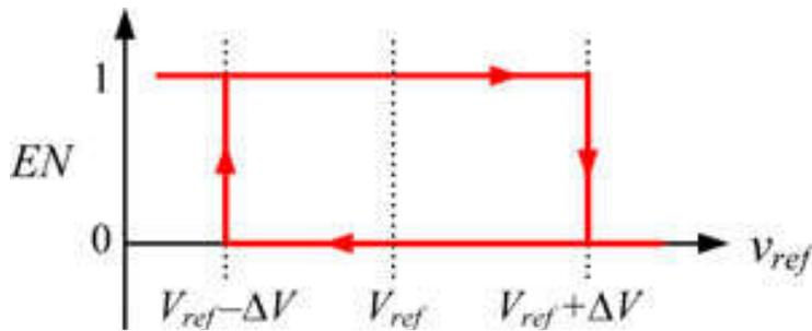
**Fig 7 Characteristics of Schmitt trigger**
