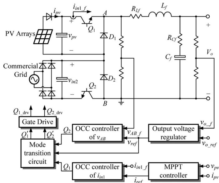
**Fig. 9 Block diagram of the whole experimental system**
